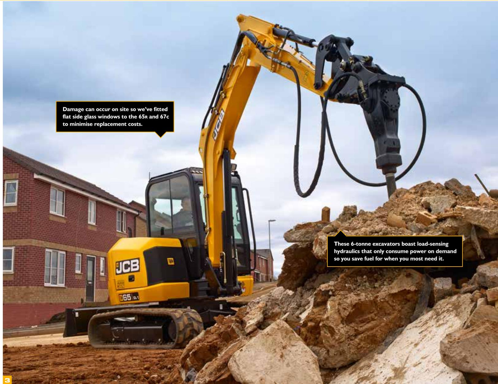
Damage can occur on site so we've fitted flat side glass windows to the 65R and 67C to minimise replacement costs.
