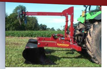
When not in use, the hydraulically operated disc marker arms can be folded back neatly behind the machine.
