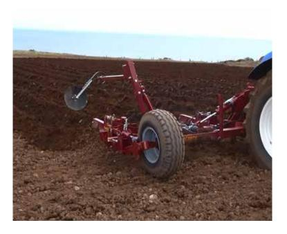
A simple and universal way of stowing the markers either when they are not in work or during road transport.
