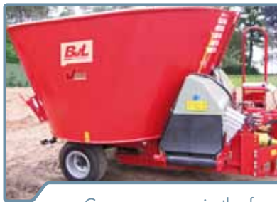
Cross conveyor in the front
