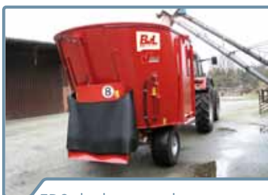
EDS discharge at the center rear
