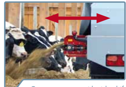
Cross conveyor with side shift
