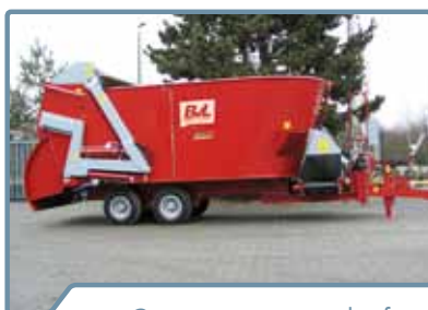
Cross conveyor in the front
