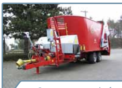
Cross conveyor in the front
