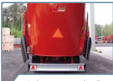
Lighting system with collision protection device
