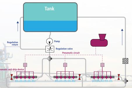
Discontinuous flow ensures that the spray mixture flows during and after spraying. Based on an AGP (Pneumatic Anti-Drip) system, it provides various advantages:
