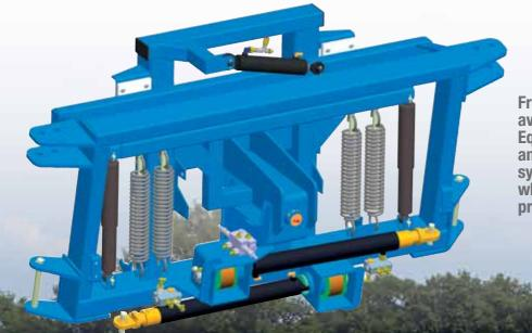
From 30m onwards, Tracker is available with the AXIALE2 boom. Equipped with an independent anti-whip device for each arm. This system reduces horizontal whiplash when accelerating and braking to protect the boom structure.
