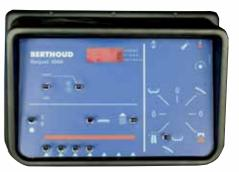
Optionally, this monitor can be used to alternately display volume/ha applied and forward speed. On demand, it can also display the litres applied, area sprayed
