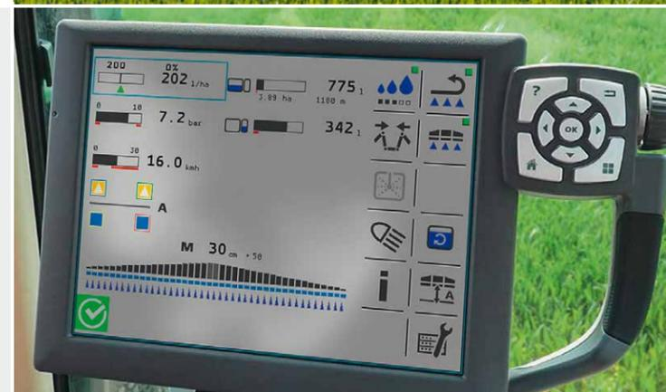
The Leeb LT can be controlled via various external terminals and joystick or the multifunction controller of the tractor.
