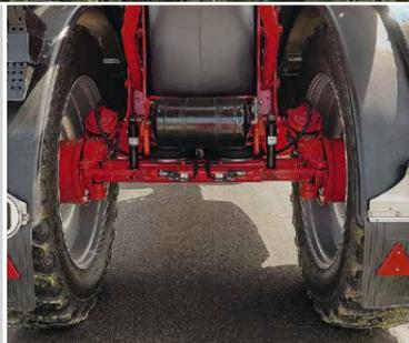
High clearance and smooth underbody with spring-loaded axle, optional: pneumatic suspension
