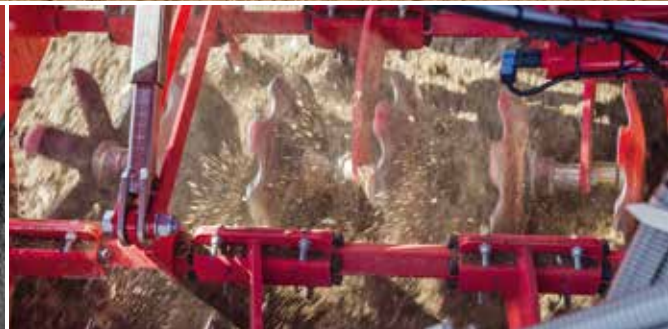
DiscSystem for intensive cultivation. Resistant even to high amounts of organic material.
