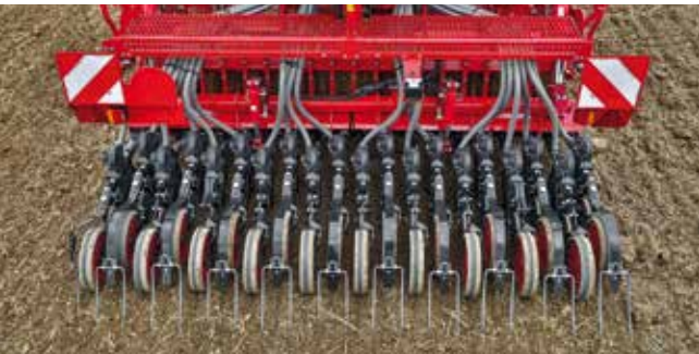
Optimum arrangement of the seed coulters behind the strip packer. One seed coulter runs exactly in the strip that has been consolidated.
