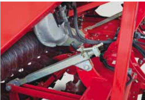
Depth adjustment DiscSystem via two adjusters. Optional: can be made while driving via two hydraulic cylinders.
