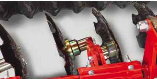
2-row DiscSystem – Considerably lower horsepower requirement compared to powered front tools (e. g. power harrow). Excellent seedbed preparation at high working speeds
