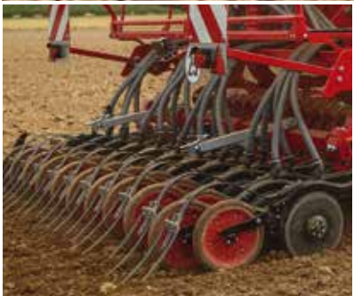
TurboDisc precision coulters of the second generation for exact seed placement even at high operational speed. In all Express TD and KR.
