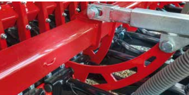
Continuous coulter pressure adjustment Manual adjustment increases the pre-stressing of the rubber elements
