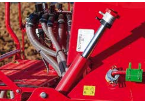
Hydraulic sowing depth adjustment with clips
