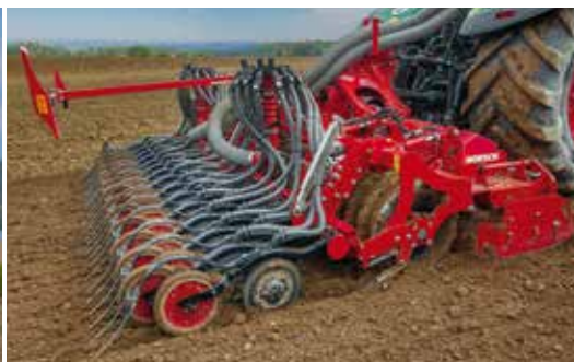
Compact unit consisting of power harrow, packer and seed coulters for a favourable weight distribution
