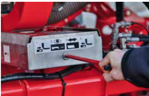
Simple and safe calibration test with a slide (opens and closes automatically) without having to reach or climb deeply into the machine
