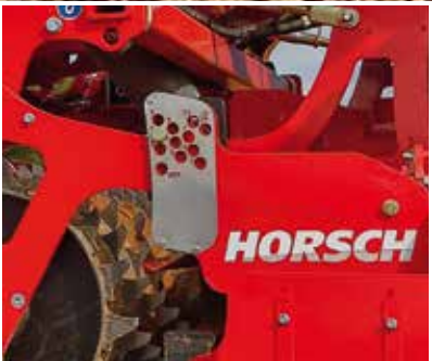
Simple and easily understandable adjustment of the working depth of the rotary harrows
