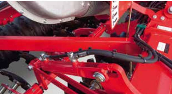
Hydraulic depth adjustment DiscSystem (optional)
