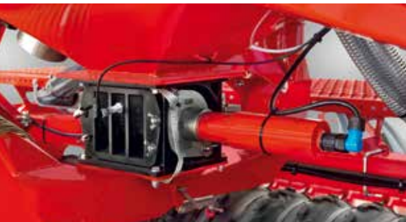
Metering unit (Express TD/Express KR) – Electric drive for metering the seed. Allows for a quick, simple and precise calibration.
