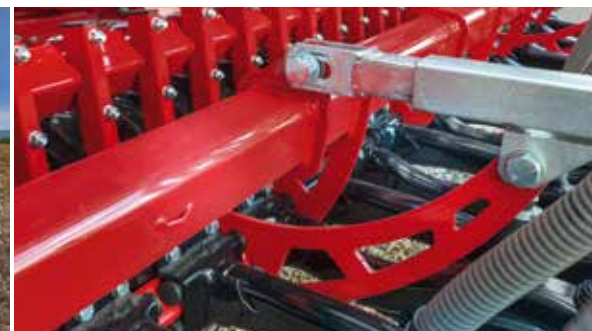
Stepless coulters pressure adjustment Manual adjustment increases the pre-load of the rubber elements
