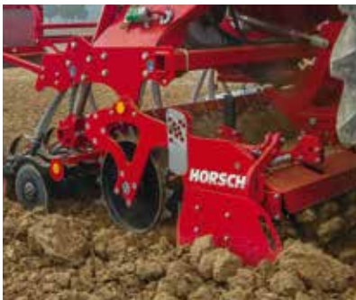
Rotary harrow Kredo crushes even rough lumps
