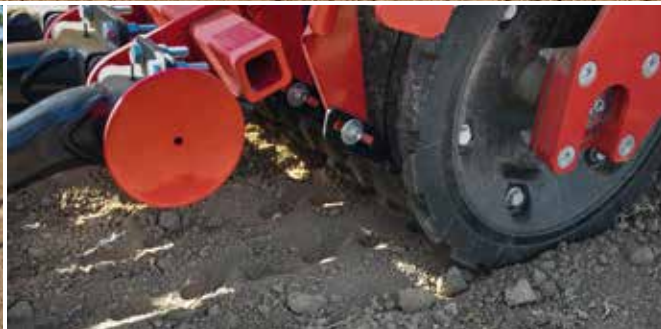
FarmFlex packer with a diameter of 54 cm for strip consolidation. It can be used on any soil.
