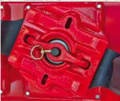
Tines with quick-change system
