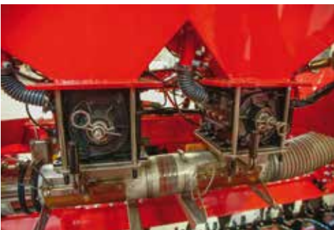
Double hopper version with the Grain & Fertilizer System (45:55)
