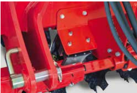
Radar sensor for an exact recording of the speed and to control the seed quantity
