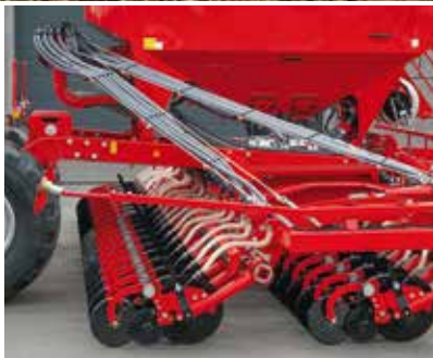
Hydraulic coulter pressure with central adjustment
