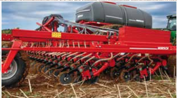
2-bar coulters design for maximum clearance
