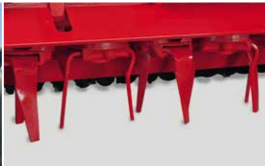
Rotary harrow Drags itself into the soil and constantly maintains the adjusted working depth.
