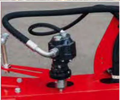
Hydraulic fan with pto-shaft drive
