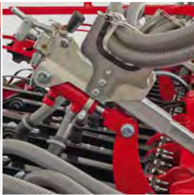
Hydraulic coulters pressure adjustment is available as an option
