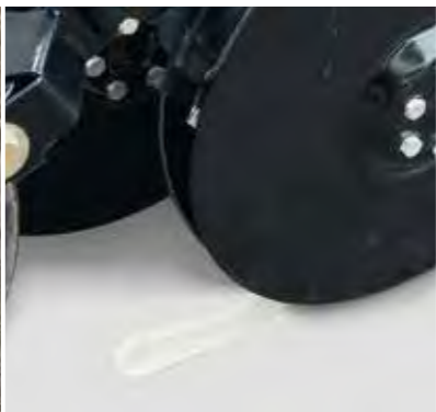
Uniformer and scraper Secure seed placement in wet conditions
