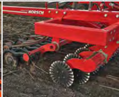
The ondulated coulters cultivate the soil efficiently and the power demand is low.
