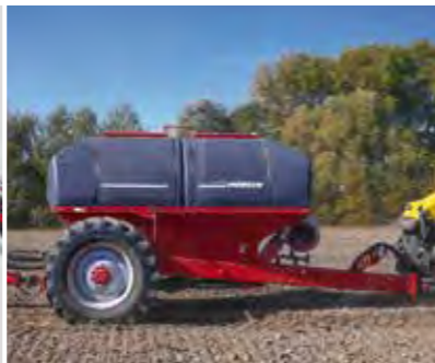
HORSCH Seed Waggon with a hopper capacity of 12 000 litre for seed and fertiliser (partition 50 : 50)
