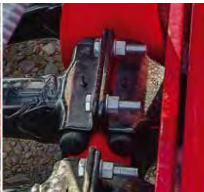
Shock absorbed mounting Good contour-following capability and overload protection
