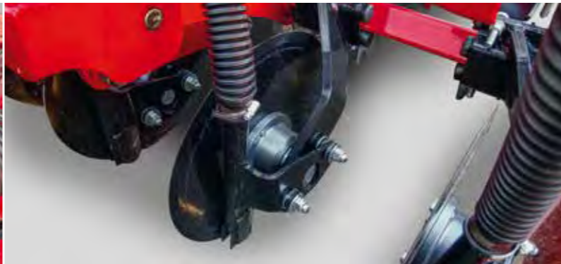
PPF fertiliser coulters Maintenance-free coulters with high coulters pressure
