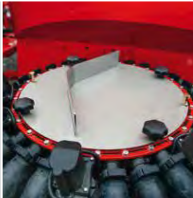
Half-width shut-off of Pronto 8/9 DC
