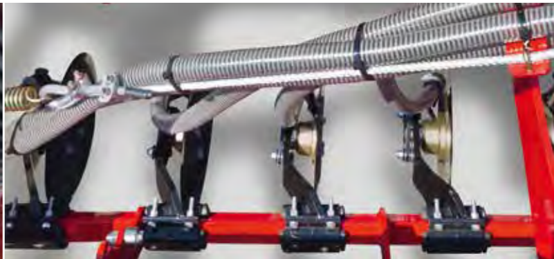
Variable depth adjustment Fertiliser placement between two seed rows, in the centre line of the tyre
