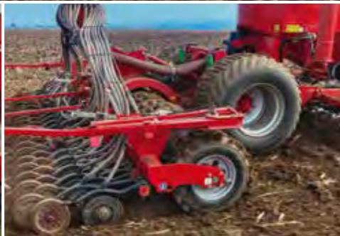
3-point linkage Quick and simple exchange of implements
