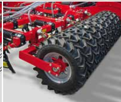
Front packer for first levelling and then improved depth control
