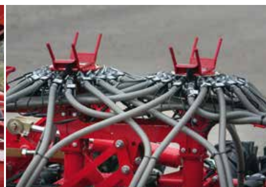
Sprinter distribution heads for an optimum cross distribution
