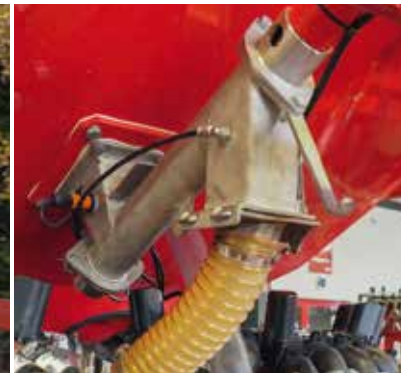
Micro-granules metered by an auger (Sprinter 3/4/6 ST)
