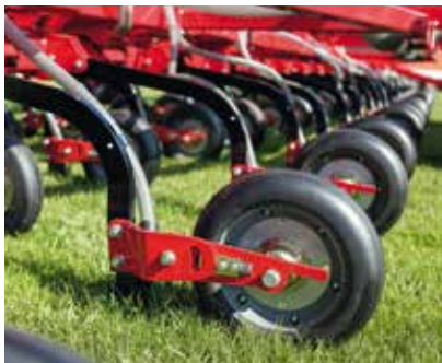
Press wheel for depth control of the seed coulters
