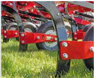
NT chisel coulters remove lumps from the seed horizon and place the grain precisely
