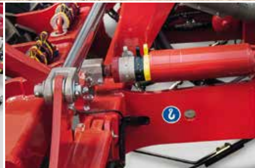
Individual depth adjustment with clip-on spacers
