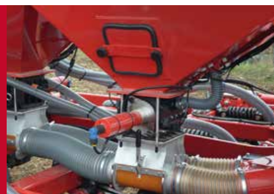
Compact metering unit Precise metering with electric drive
