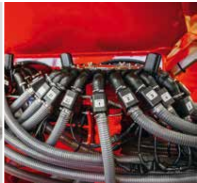
Distribution tower with tramlines valves, seed flow sensors and half-width shut-off
