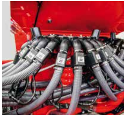
Permanent seed flow control by means of sophisticated sensor technology (optional)
