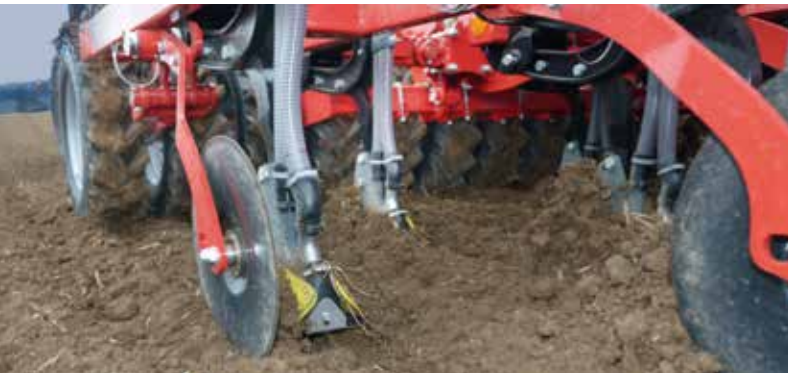
PPF fertiliser coulter – maintenance-free coulter with high coulter pressure
