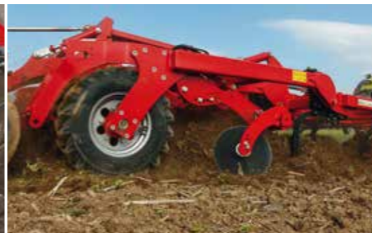
Tyre packing system Effective and deep consolidation while protecting the soil
