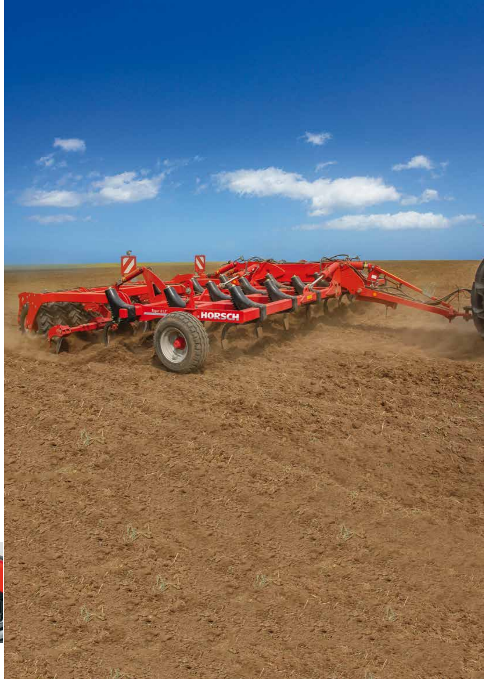
Robust tyre packing system Tyre packing system with optimised tyre thread. Suspended middle packer section serves as transport wheels for road transport.
