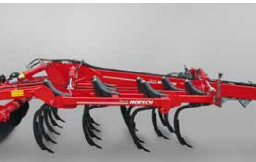
TerraGrip shank 28 cm trip height, 500 kg trip force, maintenance-free
