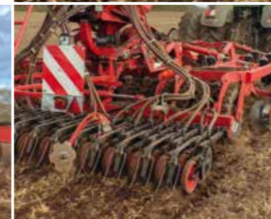
TurboDisc coulters 15 cm coulters spacing, integrated coulters suspension, variable coulters pressure of up to 120 kg/coulters
