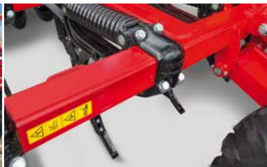
TerraGrip Release force 770 kg
