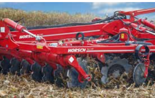
Heavy DiscSystem Arranged in two rows, disc diameter 68 cm, disc distance 40 cm, serrated discs with individual suspension
