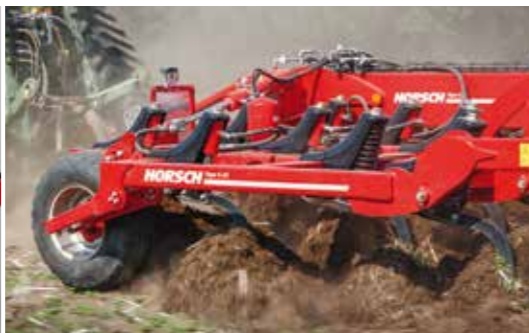
Hydraulic cylinder of the TerraGrip tine for release forces of up 770 kg (optional for first and second tine row for Tiger 5, 6, 8 AS)
