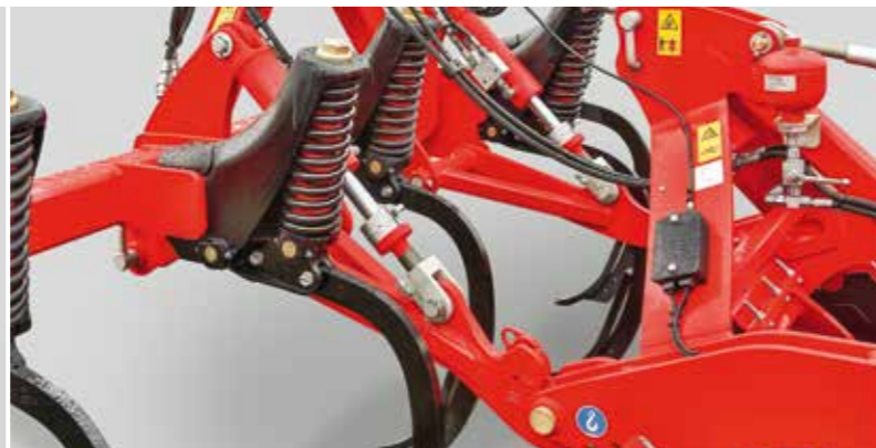
Mono TG: ideal for deep loosening. TerraGrip tines with narrow LD (low disturbance) coulter deeply loosen soil without transporting rough lumps to the surface.
