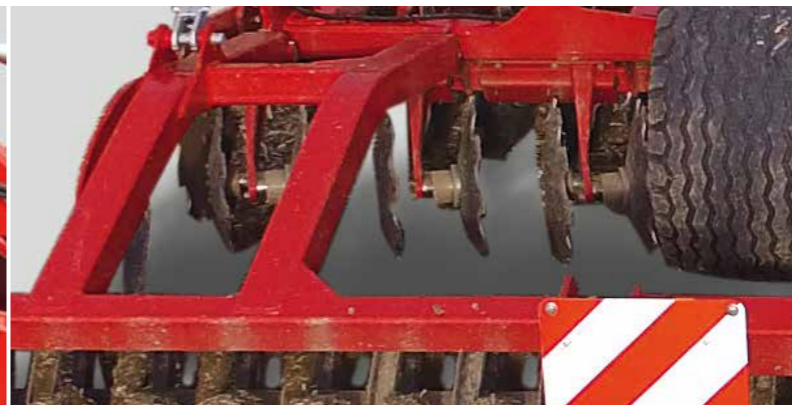
High clearance – two discs at one arm
