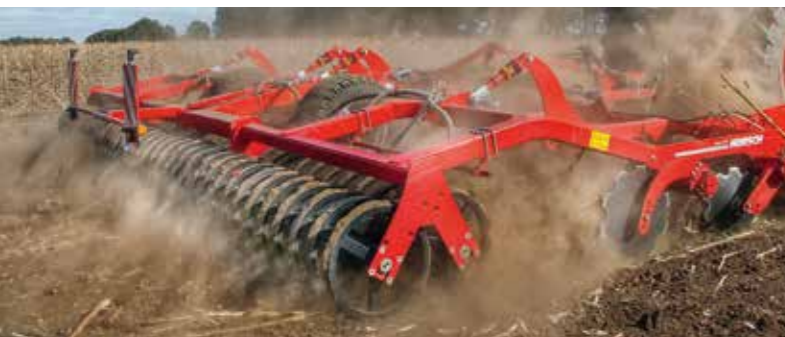
The Joker prepares a fine and consolidated seed bed with good conditions for germination
