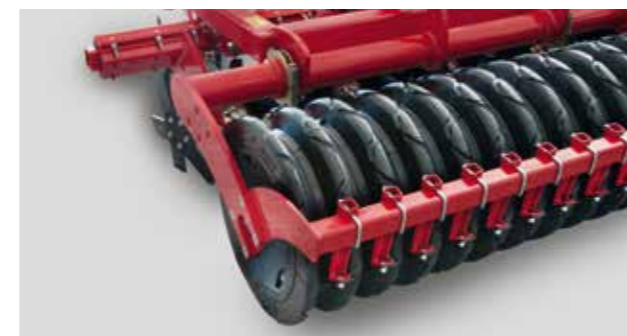
The FarmFlex packer disposes of effective and robust scrapers for trouble-free functioning
