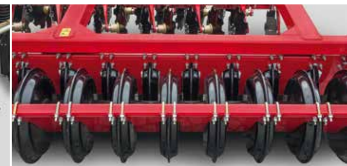
Double-SteelDisc packer for optimum consolidation even on most heavy soils
