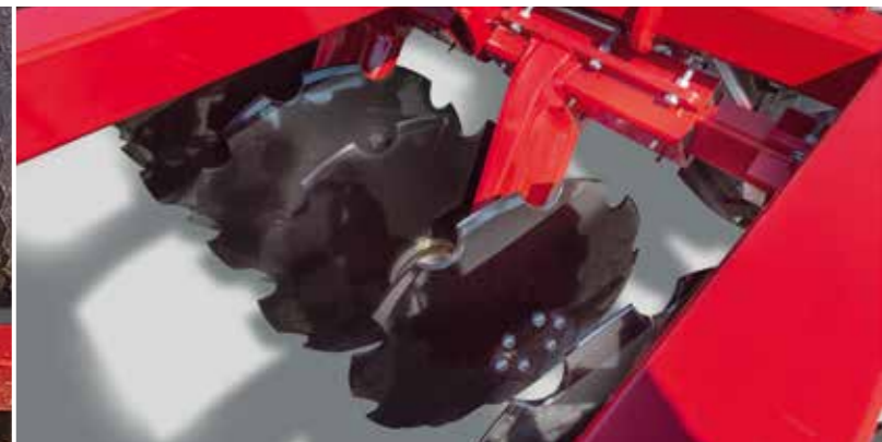
Large (Ø 62 cm) discs for working deeply
