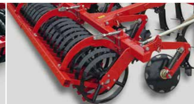
RollCut packer good surface structure on medium-heavy soils without stones
