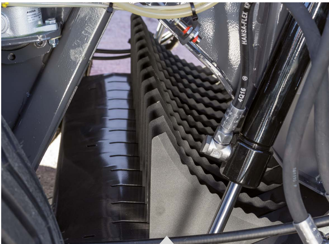
Xtracut 13 rotor features 90mm crop cutting length
