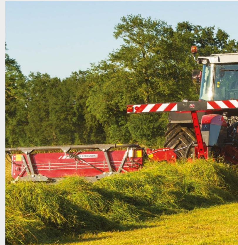
TurboLift-system (TL), which enables hydro-pneumatic discharge and continuous adjustment of pressure on the cutter bar.
