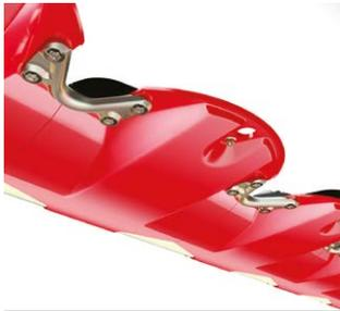
Streamline cutter bar (underside)
