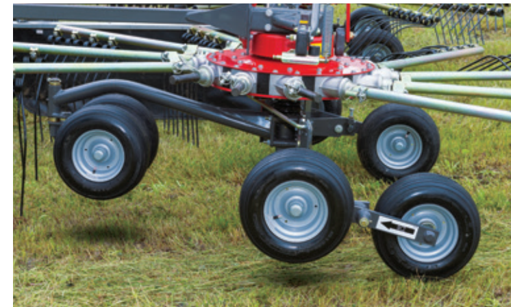
Patented, fully cardanic rotor suspension
